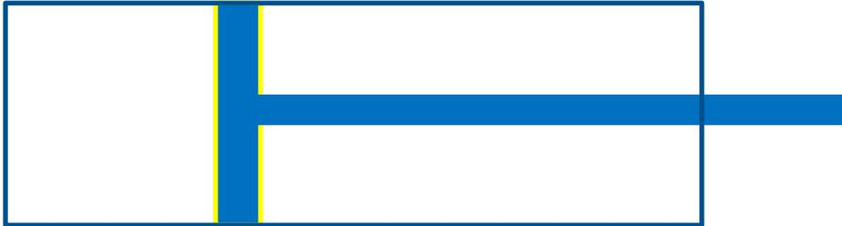
Remember that we are only concerned with the area of the plate (the highlighted yellow region) because that is the part the compressed part tries to push out to give the air more volume.
