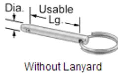
Also known as faspins, these pins have a ring grip. The ball springs inward during installation and pops out to lock the pin in place. The ball and spring are Type 316 stainless steel. The pin diameter equals the hole size. Shaft diameter tolerance is  $-0.003"$ . Shafts have a minimum Rockwell hardness of B85, except aluminum have a minimum Rockwell hardness of B56. Breaking strength is measured as single shear, which is the force required to break a pin into two pieces.
