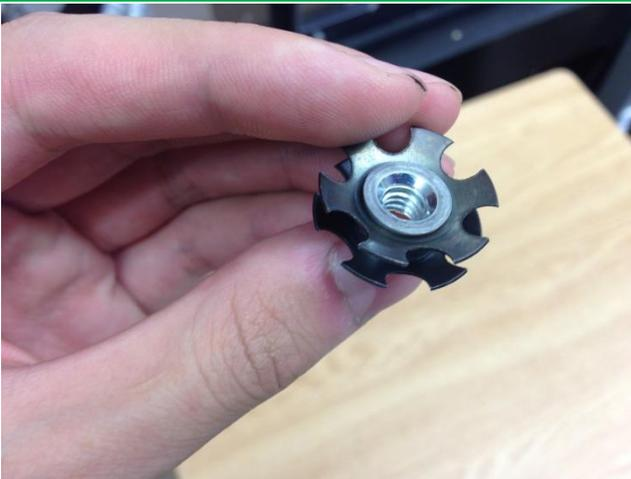
Quite simply, these are shoved into the ends of round tubes. To connect the end of the tube perpendicular to something, pound the insert into the end of the tube, and secure a perpendicular plate to the end by putting a screw through it. (This works similarly to how a base flange works for a pipe.)
