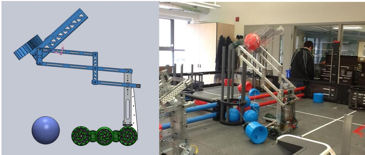
Here is a VEX robot made out of custom parts. Its lift uses a 6-bar linkage. Basically, it is a clever series of joints that keeps the end (the tray) parallel to the ground as the tray moves up and down. If it were just a single pivot and the tray was fixed to the arm, the tray would change angle relative to the ground as the arm moves up and down.
