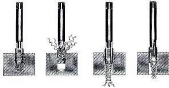
To tap a hole; first drill a hole slightly smaller into the part, then turn the tap into the part as if you were screwing it in.
